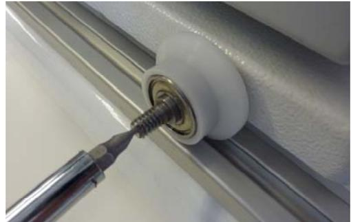
Remove the right front and back wheel (viewed from the front). Install the EdgeRider wheel with the sliding hub (pictured to the right) using the 1-1/4" bolt and two thick washers between the sleeve and the machine and 1 thin washer on the outside of the wheel.
