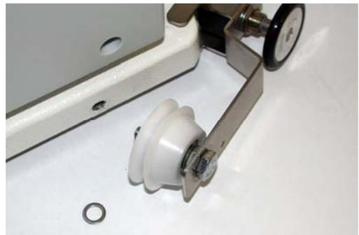
Mount the wheel/sensor assembly on the machine. Tighten the bolt, so the back of the locknut holds the wheel firmly. Check the looseness of the bracket and adjust the locknut if necessary.
