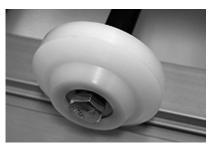
If there was an "L" bracket on the left front wheel, reinstall it, but put two washers between the bracket and the wheel to provide safe clearance.
