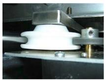
Install the wheels on the front using the 1-1/2" bolts. MAKE SURE THAT YOU PUT ONE LARGE WASHER ON THE TOP AND ONE SMALL WASHER ON THE BOTTOM OF EACH WHEEL. Put any additional/original washers/spacers on the top of the wheel. If you have the eccentric bolts, turn them to the widest position. If there is a slot provided for adjustment, push the bolt gently toward the table.
