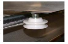
Install the wheels on the front using the 1-1/2" bolts. MAKE SURE THAT YOU PUT ONE LARGE WASHER ON THE TOP AND ONE ON SMALL WASHER THE BOTTOM OF EACH WHEEL. Put any additional/original washers/spacers on the top of the wheel. If you have the eccentric bolts, turn them to the widest position. If there is a slot provided for adjustment, push the bolt gently toward the table.
