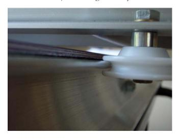
EdgeRider Wheels Installation Manual for APQS Machines with New Channel Locks the wheels as described above. Use the 1 3/4 inch bolts.
