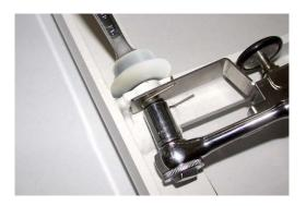
Install the remaining non-sliding hub wheel on the other side of the front of the carriage, using a 1-1/4" bolt, putting two thick washers between the wheel and the carriage and 1 thin washer on the outside of the wheel.
