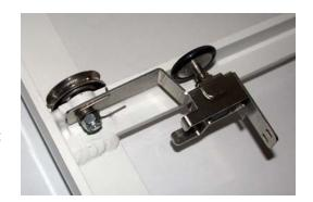
Drive the bolt into the threaded hole on the carriage. Mount the washers, the spring and the lock nut in their original order. Hold the bolt from turning and tighten the locknut enough to keep the bracket aligned, but freely moving.
