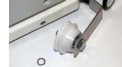
Remove the right front and back wheel. Install the EdgeRider wheel with the sliding hub (pictured to the right) using the 1-1/4" bolt and one thin washer between the sleeve and the machine.
